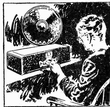
A Master Station Selector, with illuminated dial for shadowy corners, enables tuning for ordinary reception with a single tuning knob.
